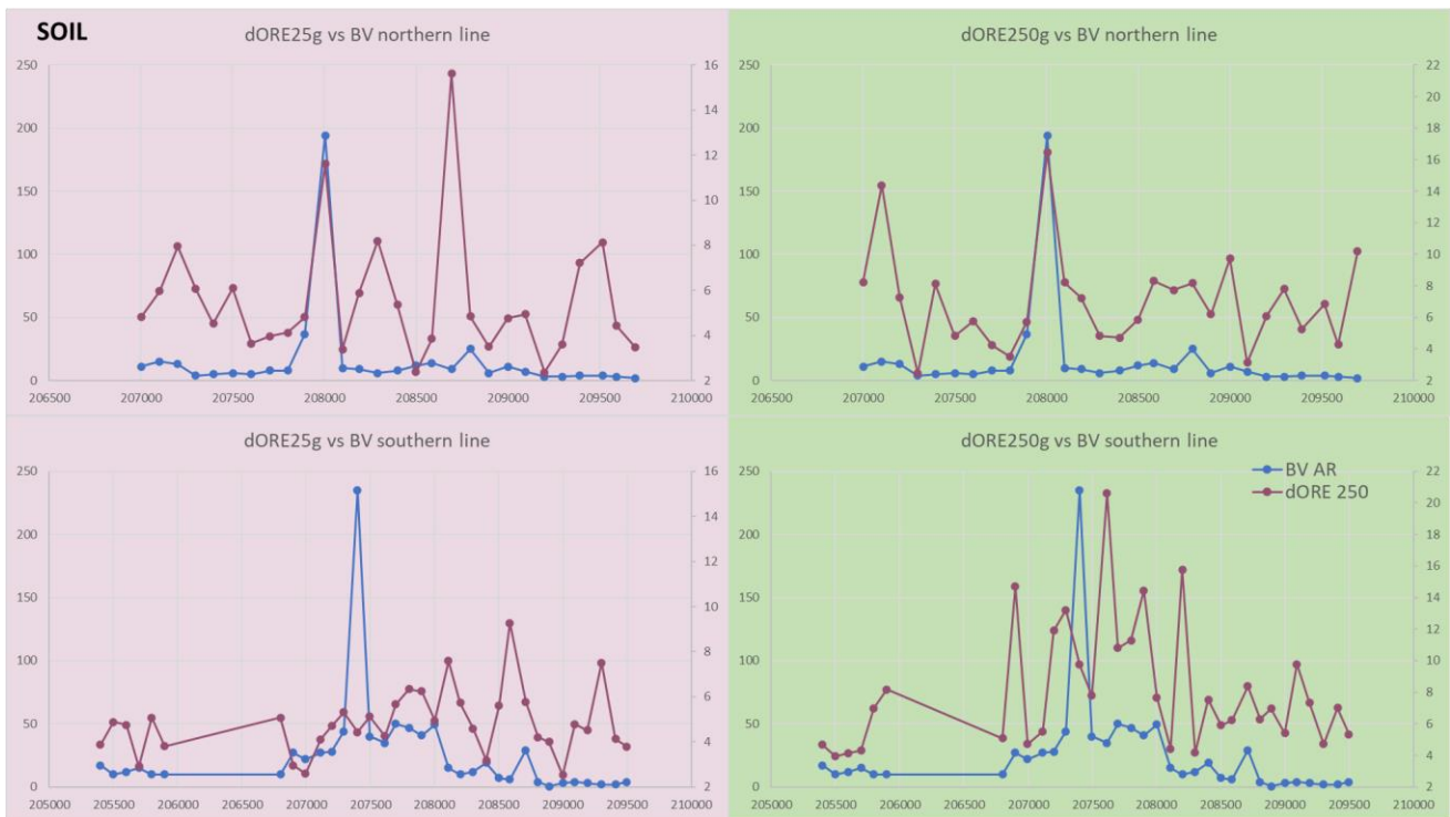
Figure 73: Line plots of the soil sample data shown in Figure 71. The left hand axis is for the aqua regia data (ppb Au) and the right hand axis is the dF value recorded by detectORE™.
